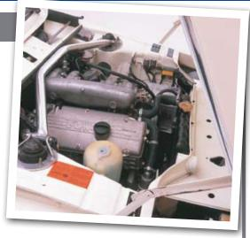
If a single-carb engine runs badly and doesn't seem to respond to tuning, then the throttle spindle may well be suffering from play - the throttle bodies have a tendency to wear and fixing the problem involves machining and a new spindle. An upgrade to twin carbs is probably cheaper.
