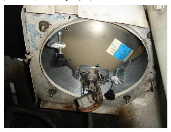
Adjust unit in correct position so grill doesn't foul unit and the lamp is central (where you previously marked it).
