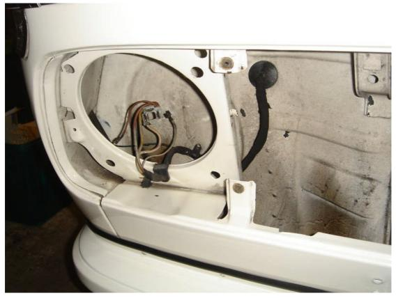
Before fitting new unit it is easier to refit the bulbs (or new bulbs) then offer up new unit to panel and hold in place whilst bolting loosely into place.
