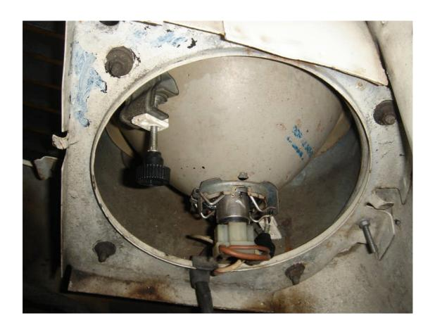
Ease plug off main bulb and side light below main bulb and pull wires out the way. Mark from the front position of old unit so new unit will go exactly in the same place. You can now gain access to the nut holding the grill in the front panel. Loosen all four 8MM nuts, don't let old unit drop out the front and when refitting new unit. Lift old unit away and store out the way.
