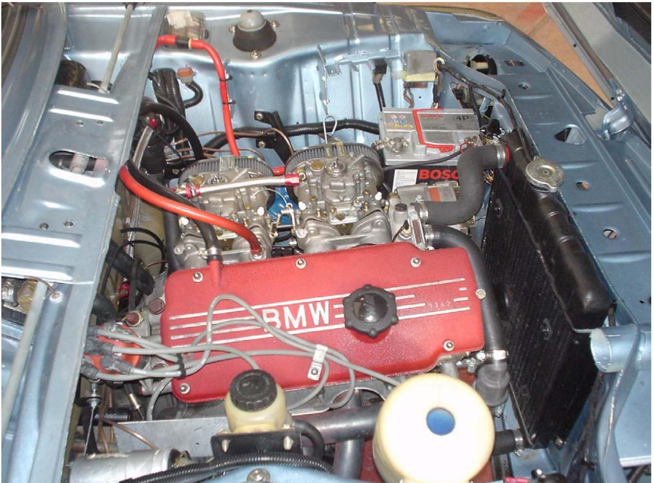
*Typical Twin Carburettor set-up*
